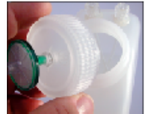
The bottle has an air filter to let air in and keep dust out.
